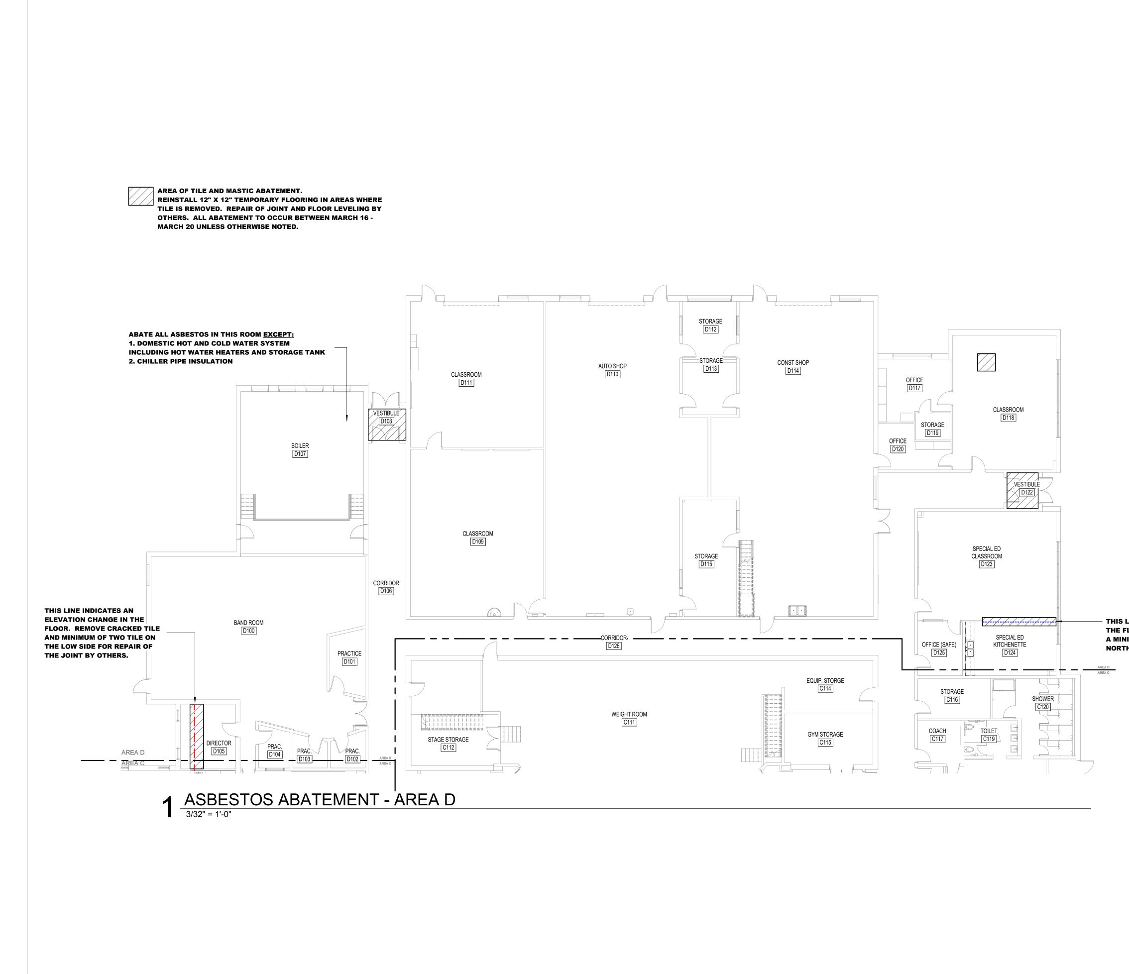
THIS LINE INDICATES CRACKED TILE IN THE FLOOR. REMOVE CRACKED TILE AND A MINIMUM OF ONE WHOLE TILE ON THE NORTH SIDE OF THE JOINT.
